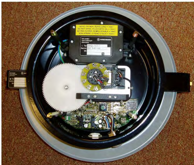
CAN-Bus electronics in cable reel.
