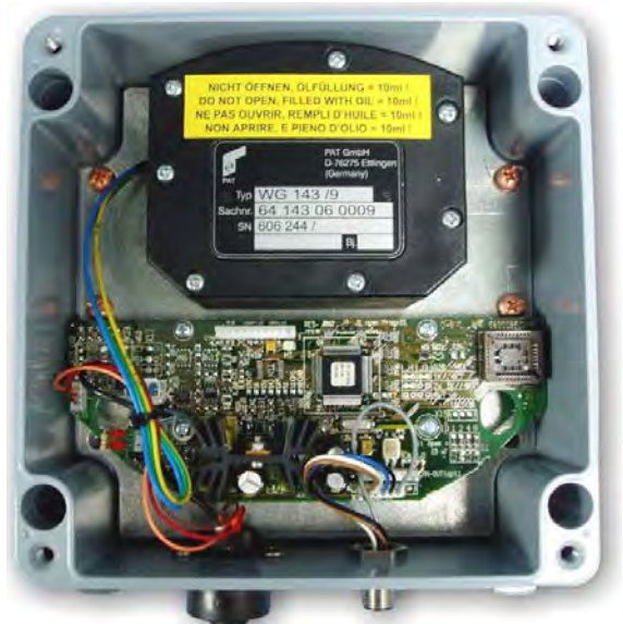
CAN-Bus electronics in angle sensor box.
