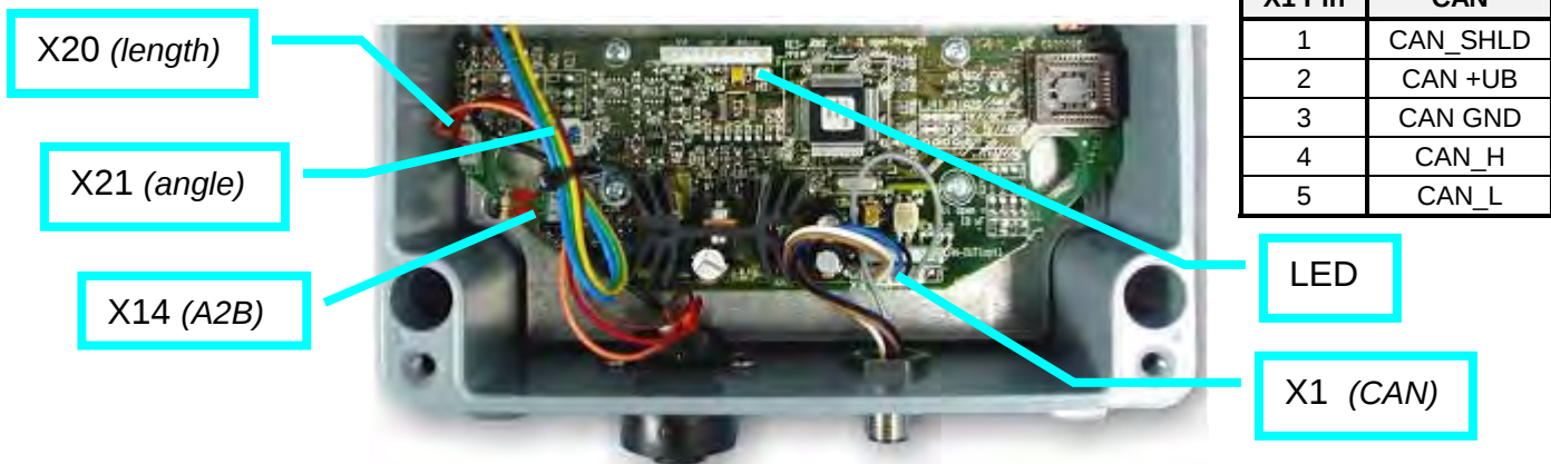
CAN-Bus electronics in angle sensor box.
