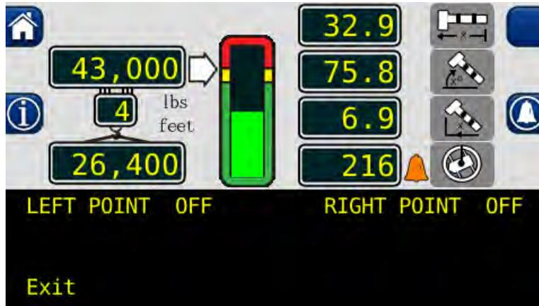
5. Rotate the boom to the desired left point. This should be the point to the left of the obstacle facing the exclusion zone to be defined.
