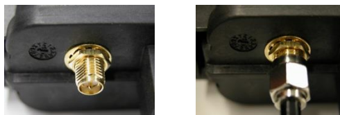
Connecting Antenna to TRS10-W2
