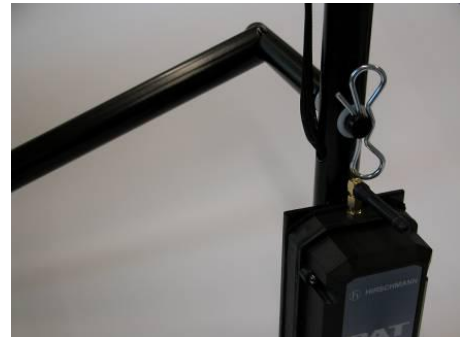
Figure 5: Mounting Tube with Sensor Mounted
