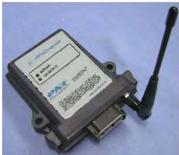
031-300-060-596 TRS 05 REPEATER 031-300-050-688 ANTENNA, 918 MHz RCL 90°
